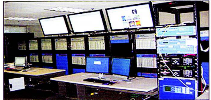
Fig. 2. Simulation software and real-time digital simulation hardware
