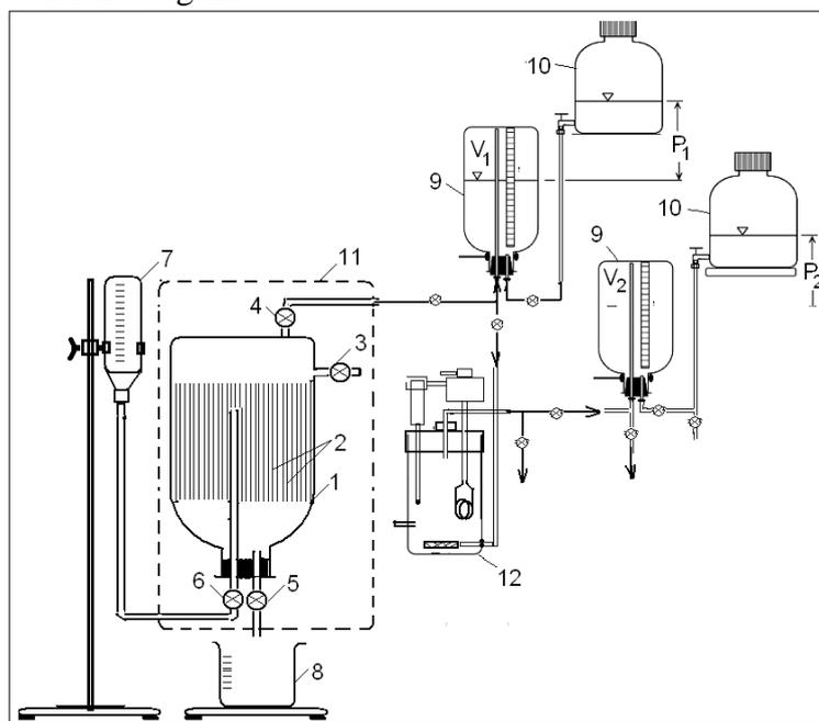
**Fig. 1.** The scheme of bench-scale reactor for biochemical generation of biogas and its purification from the admixtures:
