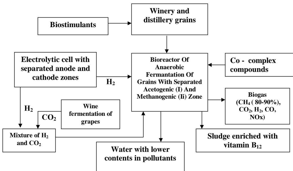
**Fig. 2.** Scheme of intensified anaerobic treatment of winery grains with the enhanced biogas yield
