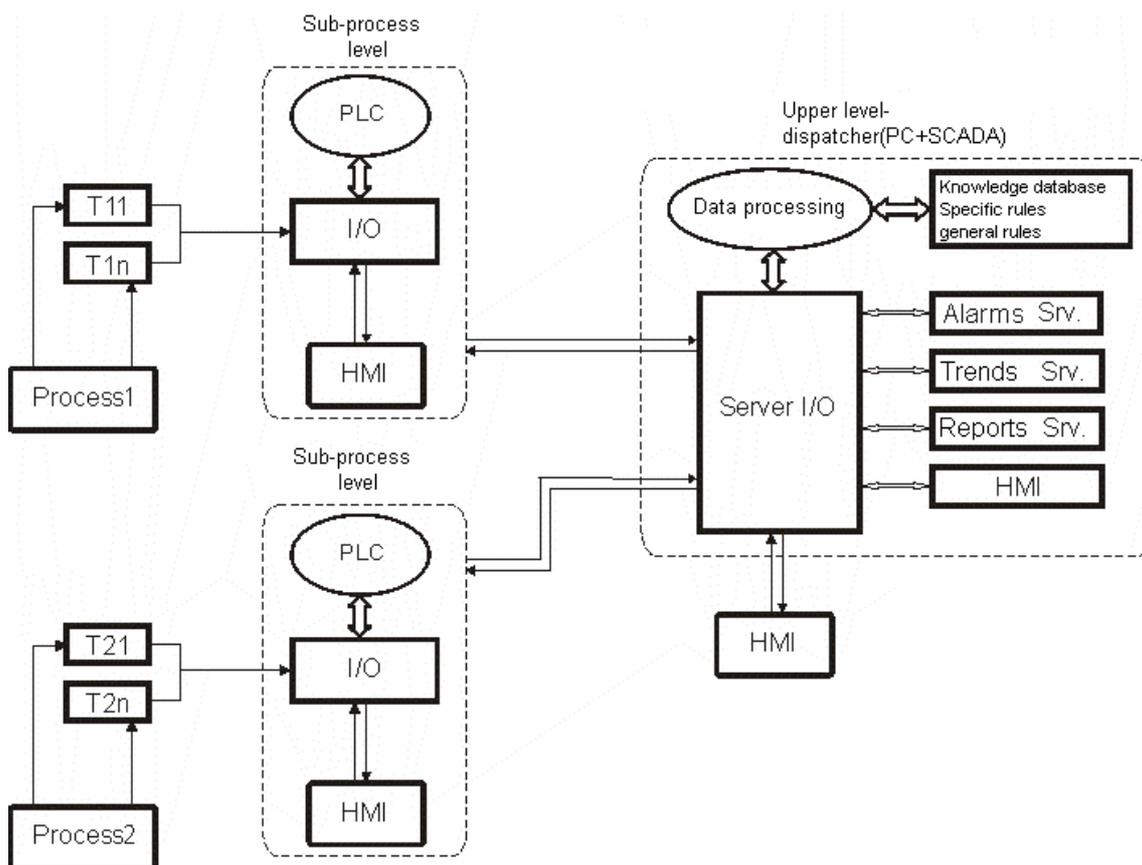
Figure 2. Hierarchically monitoring system distributed on two levels.
