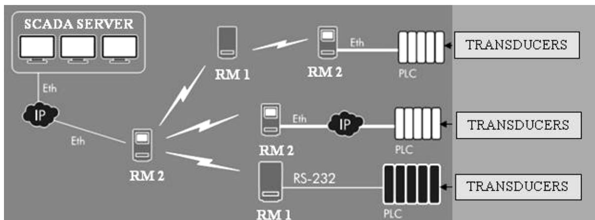
Figure 1. Wireless data transmission to a SCADA server using radio modem equipments.
