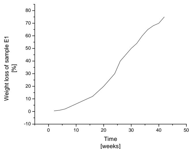
Figure 1. The weight loss variation of sample E1, sample with thickness 0.140 mm.
