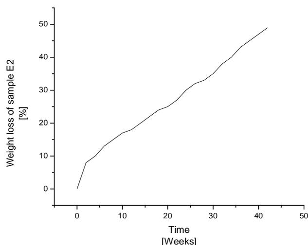
Figure 6. The weight loss variation of sample E2, sample with thickness 4 mm.
