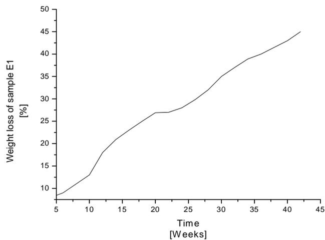
Figure 5. The weight loss variation of sample E1, sample with thickness 4 mm.
