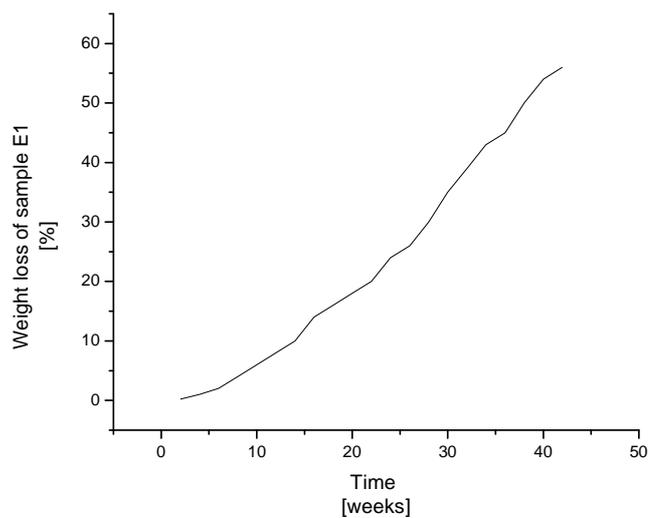
Figure 3. The weight loss variation of sample E1, sample with thickness 1 mm.
