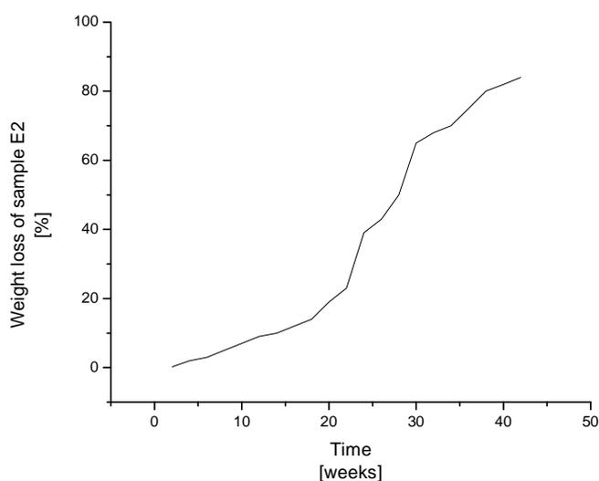
Figure 2. The weight loss variation of sample E2, sample with thickness 0.140 mm.
