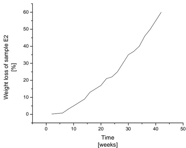
Figure 4. The weight loss variation of sample E2, sample with thickness 1 mm.
