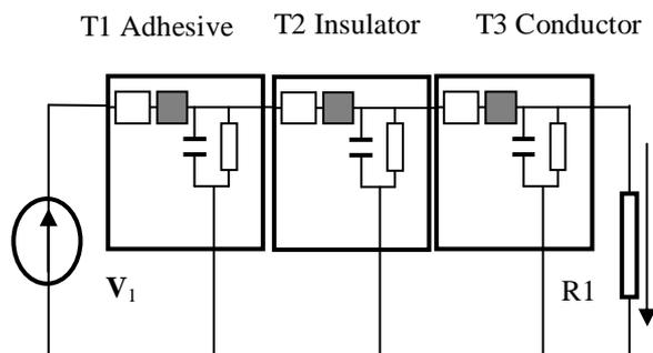
Figure 3. Layered composite material transmission line model.
