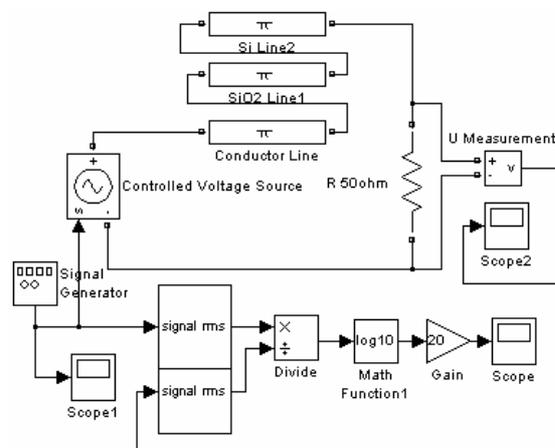
Figure 5. SIMULINK simulation model for composite material.
