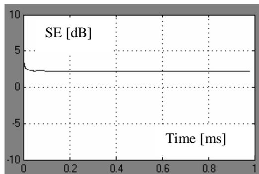
Figure 6. The shielding effectiveness simulated at 10 GHz.
