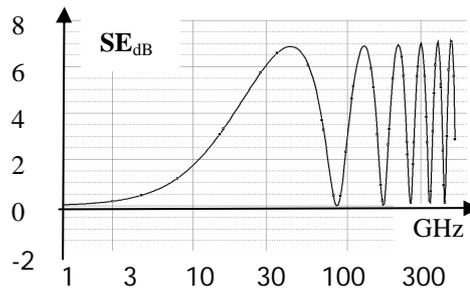
Figure 4. The material attenuation in the frequency range of 1GHz - 500GHz.
