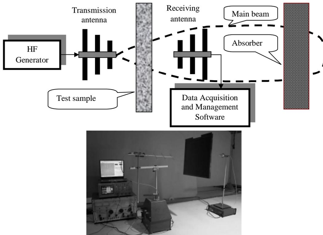
Figure 8. The composite material sample positioned between the transmitter and reception antennas.
