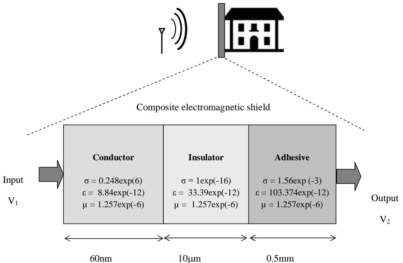
Figure 2. About the composite material structure.
