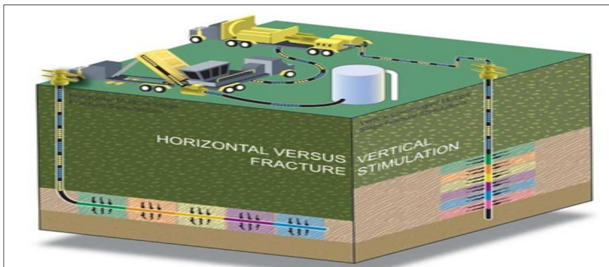
Figure 3. Vertical versus horizontal drilling.
