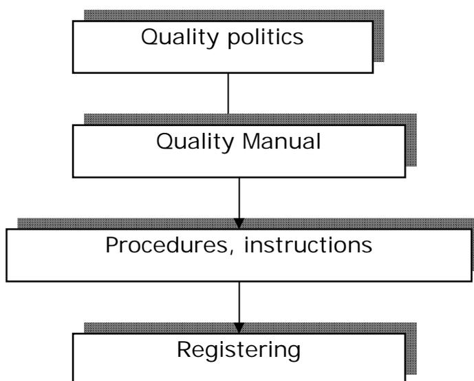
Figure 1. Elements of the quality system for laboratory.
