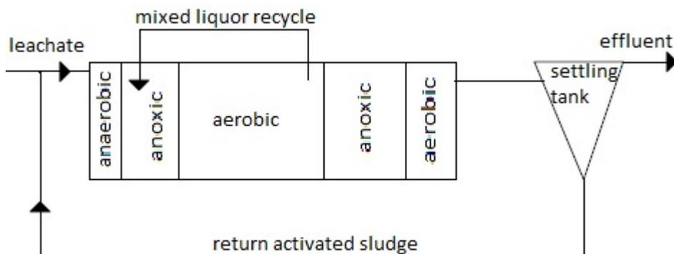
Figure 2. Bardenpho scheme for nutrient removal.
