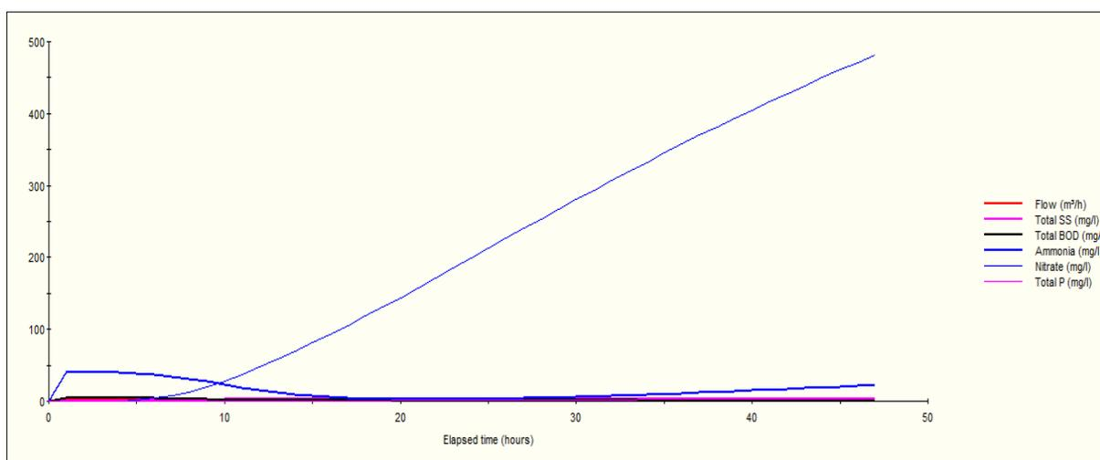
Figure 6. Results for total suspended solids, BOD, ammonia, phosphorus and nitrates removal using Bardenpho scheme.
