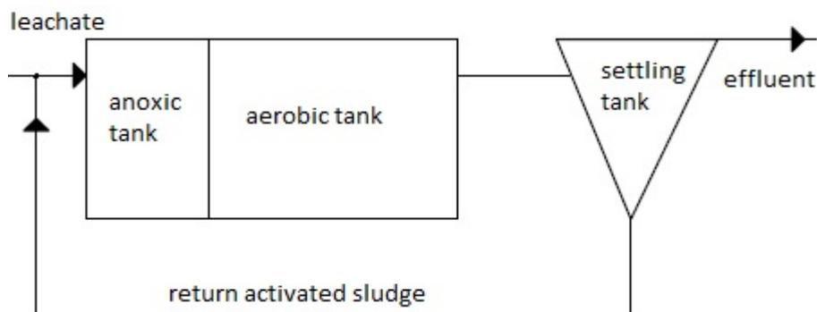
Figure 1. AO (anoxic-oxic) scheme for nutrient removal.
