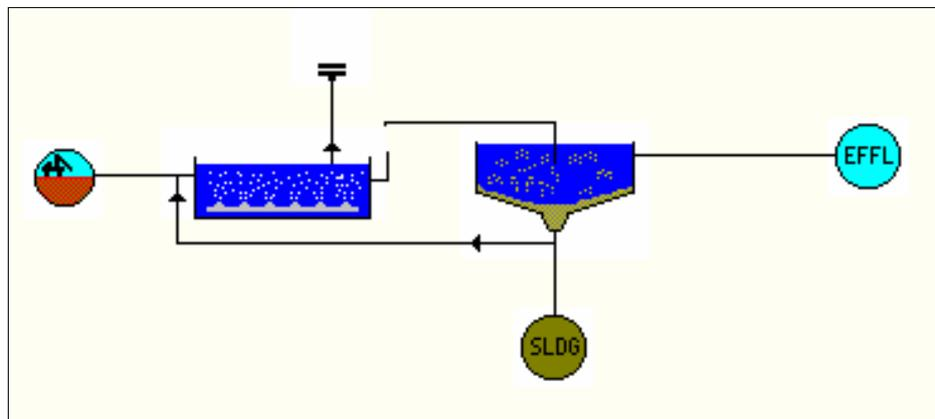
Figure 3. STOAT model for nutrient removal schemes.
