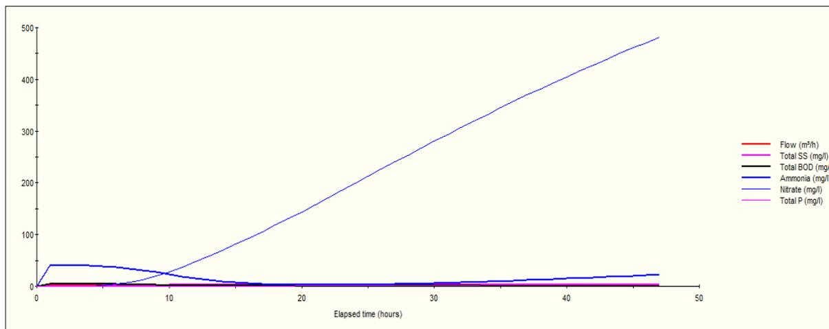
Figure 5. Results for total suspended solids, BOD, ammonia, phosphorus and nitrates removal using AO scheme.
