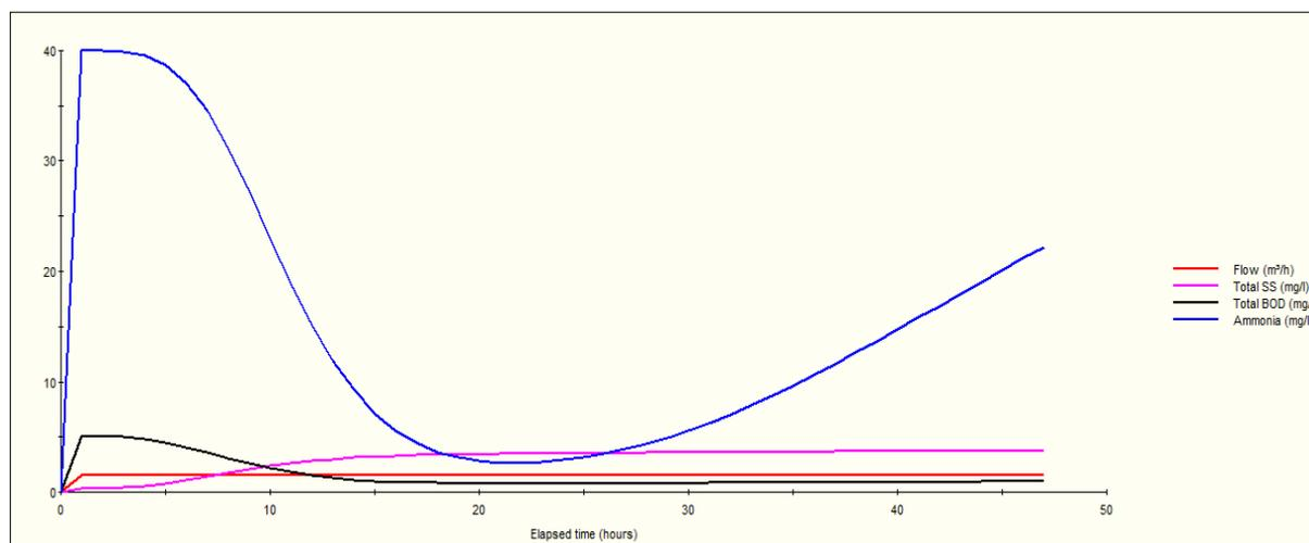
Figure 4. Results for total suspended solids, BOD and ammonia removal using AO scheme.
