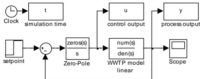
Figure 6. PID control of the process. Linear process model.
