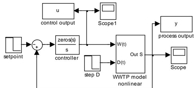
Figure 7. PID control of the process. Nonlinear process model.
