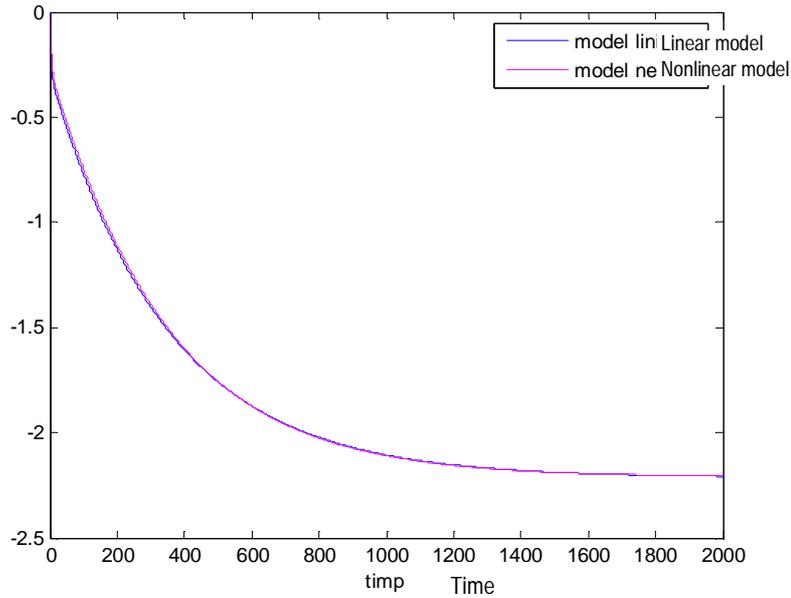
Figure 5. The step response of the systems for perturbation  $D = 0.15$ .
