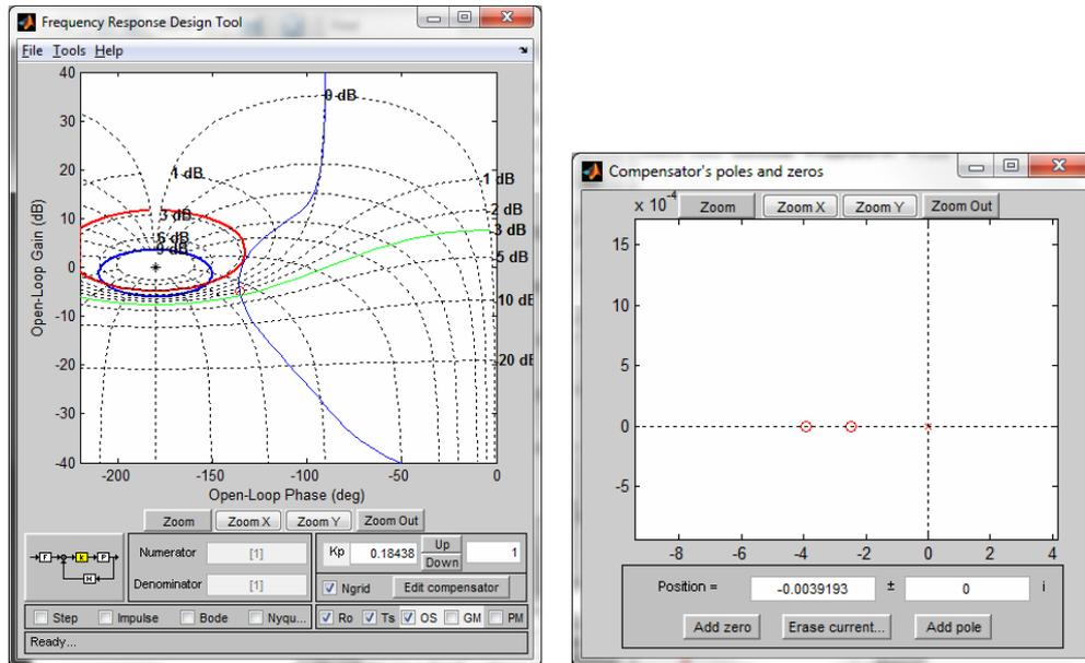
Figure 3. PID design with FR-tool.
