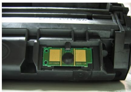
Figure 2. Chip mounted on the cartridge.
