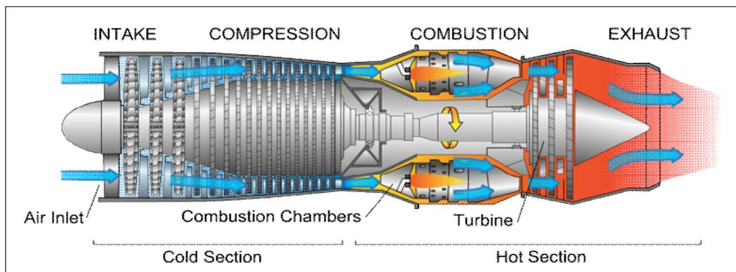
Figure 1. Turbojet engine components (Hunecke 2010).
