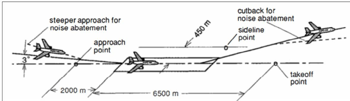
Figure 2. FAR part 36 - noise certification requirements (Kerrebrock 1992).
