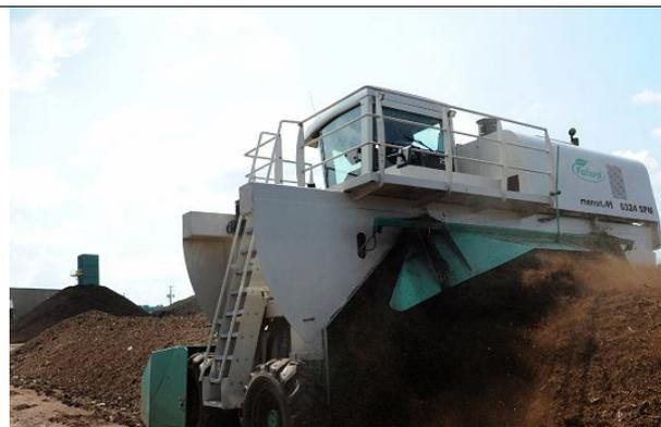
Figure 2. Aeration equipment used in composting (Source: Fafard et Frères 2013).
