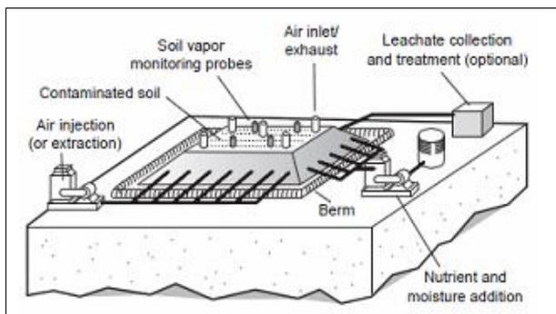
Figure 5. Typical Biopile Setup
