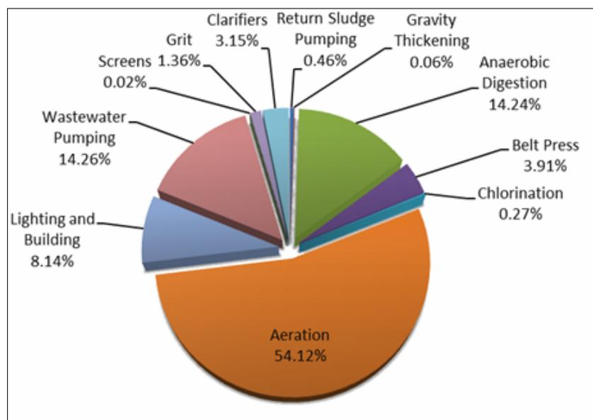
Figure 1. Total energy consumption use for a wastewater treatment plant (erc.uic.edu).
