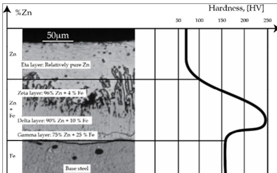
Figure 1. Hot dip galvanized coating composition (Marder 2000; Reumonta et al 2001; Shibli & Manu 2006; Sistonen 2009).
