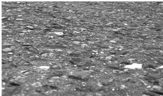
Figure 3. Asphalt-containing waste glass (Huang et al 2007).
