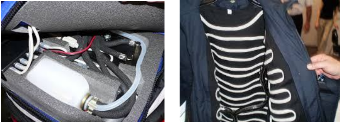
Figure 3. The circulation of liquid that is cooler than the environment in tubing built into clothes (Source: Thermofalsh Kft. 2010).
