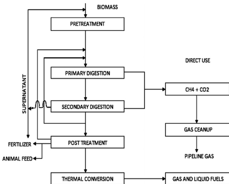
Figure 1. Scheme of anaerobic digestion (Tock et al 2010).
