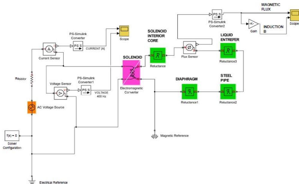
Figure 6. The SIMULINK model for checking up the magnetic mode.
