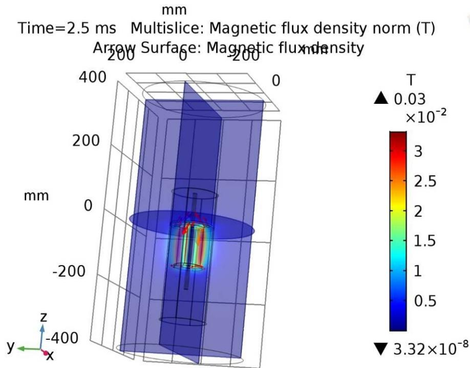
Figure 5. The intensity of the magnetic flow inside the magnetic module – a 3D model.
