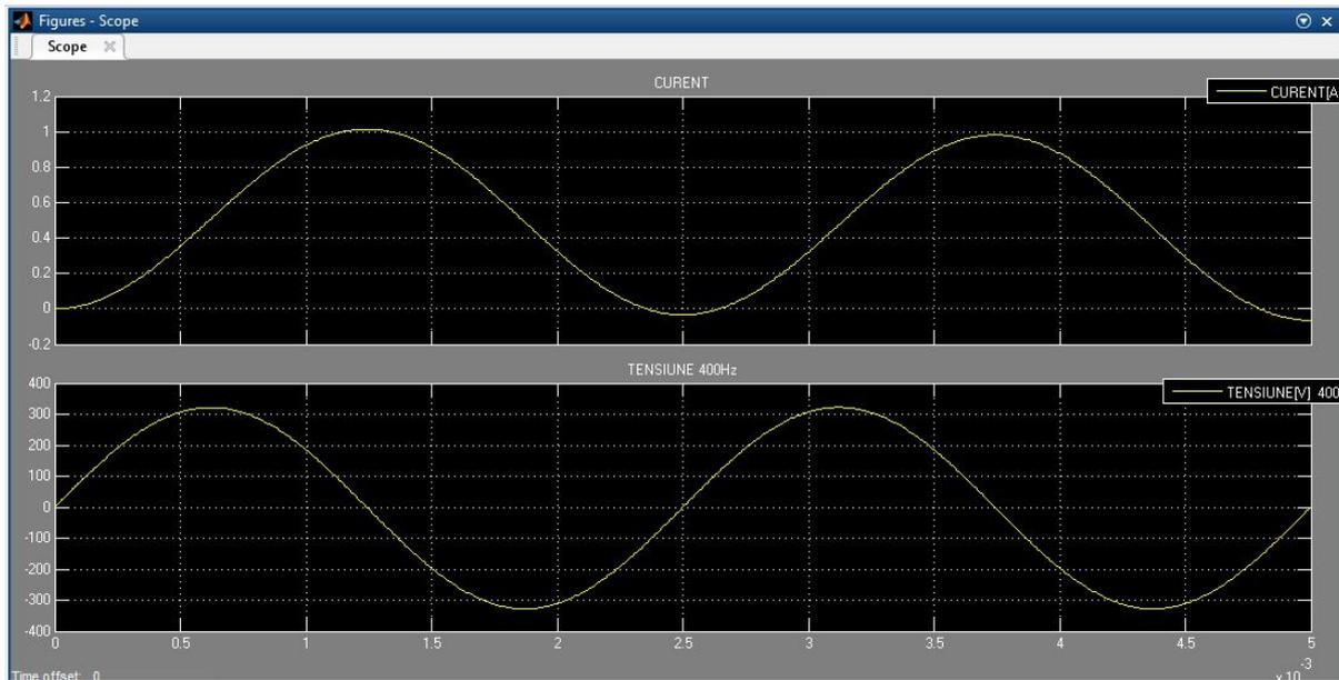
Figure 7. The solenoid supplying voltage and current – the SIMULINK model.
