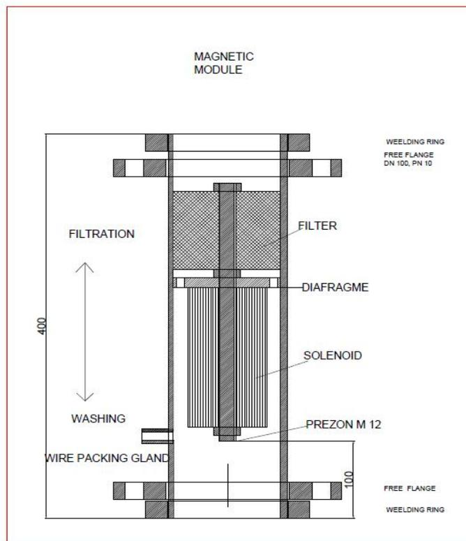
Figure 2. Theoretical drawing for the magnetic module.
