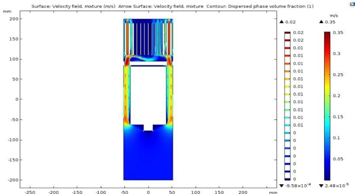
Figure 3. The simulation of the water flowing rates in the magnetic module, obtained by means of the COMSOL software.
