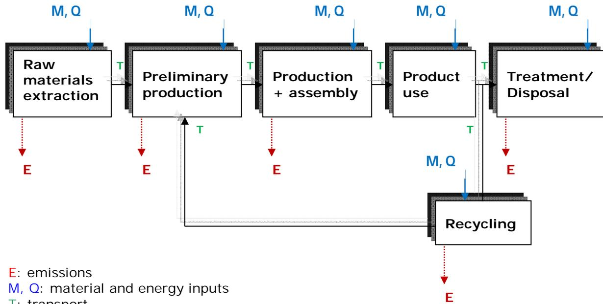
Figure 1. General life cycle of a photovoltaic system.
