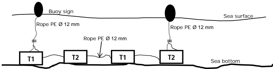
Figure 4. Design of 1 series of attractor setting in the waters.
