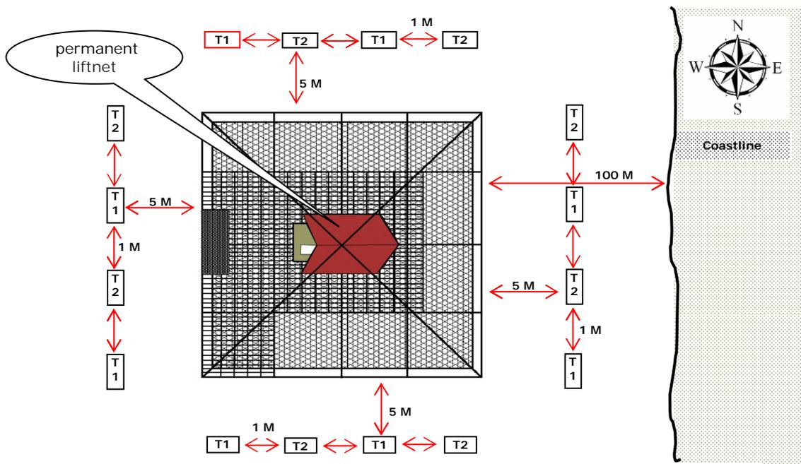
Figure 5. Design of squid attractor setting around liftnet.
