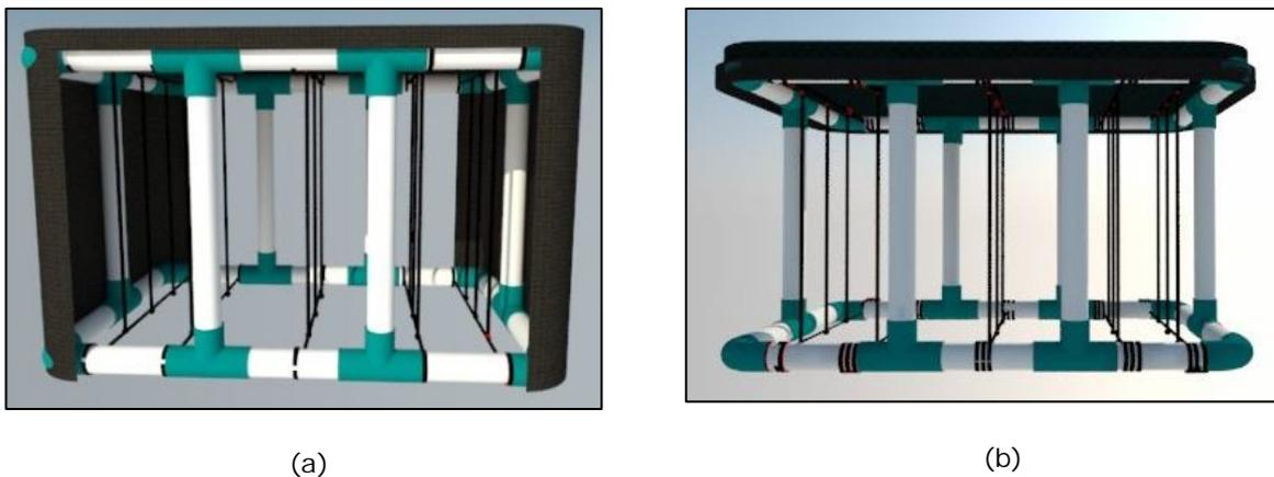
Figure 3. Squid attractor; (a) Type 1 (T1) with cover net (Polyethylene 40%) on the upper and both sides and (b) Type 2 (T2) with cover net (Polyethylene 40%) only on the upper side.
