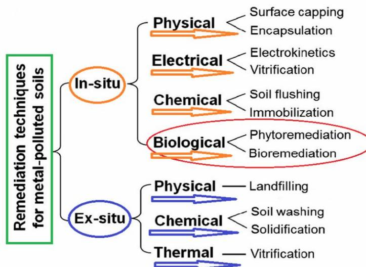
Figure 3. Remediation methods for heavy metal-contaminated soils.
