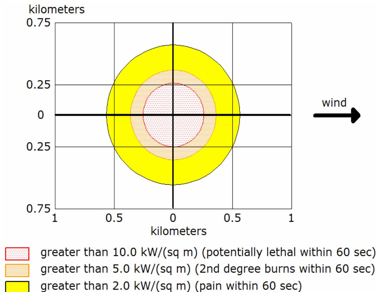
Figure 4. The standard areas of danger according to ALOHA software.
